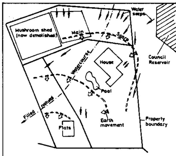
Figure No.8 - Bowral Landslip Mechanism
