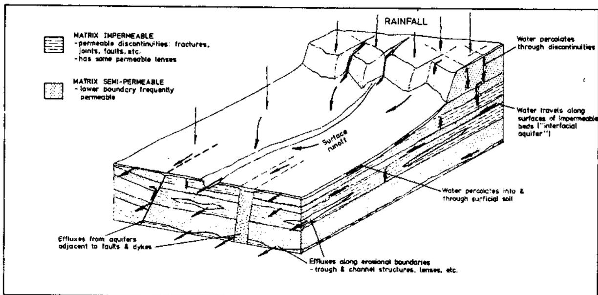
Figure No.2 Geological Control of Groundwater Flow
