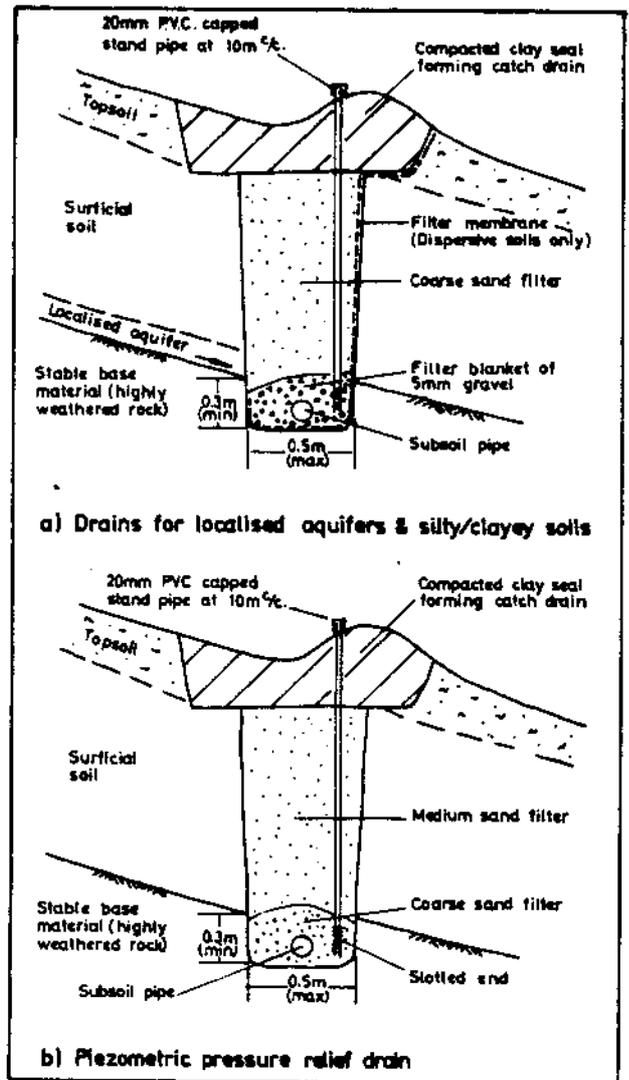
Figure No.4 - Typical Interceptor Drains
