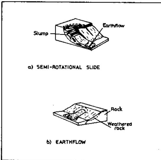
Figure No. 1 - Landslide Mechanisms
