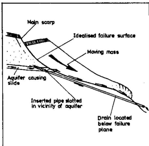
Figure No.5 Typical Inclined Drains
