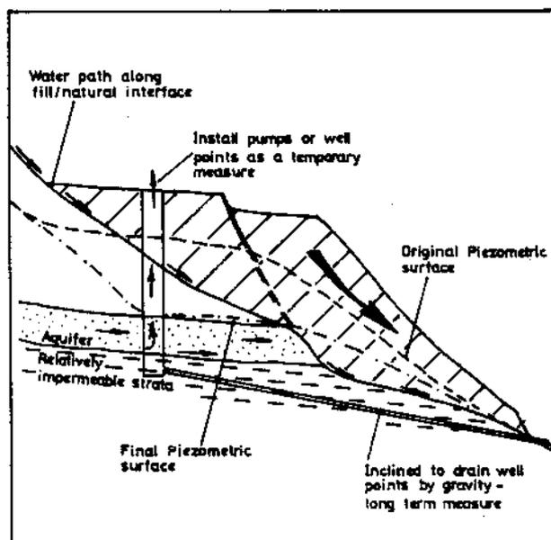
Figure No.6 - Typical Gravity Drainage Well
