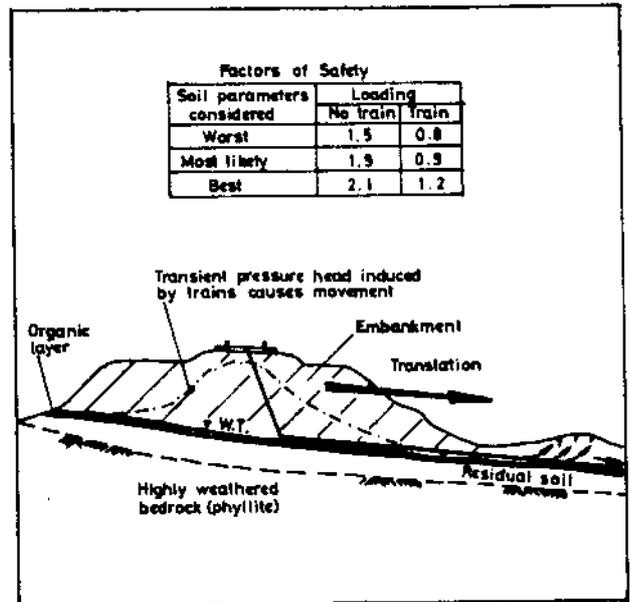
Figure No.11 - Newee Creek Failure Mechanism
