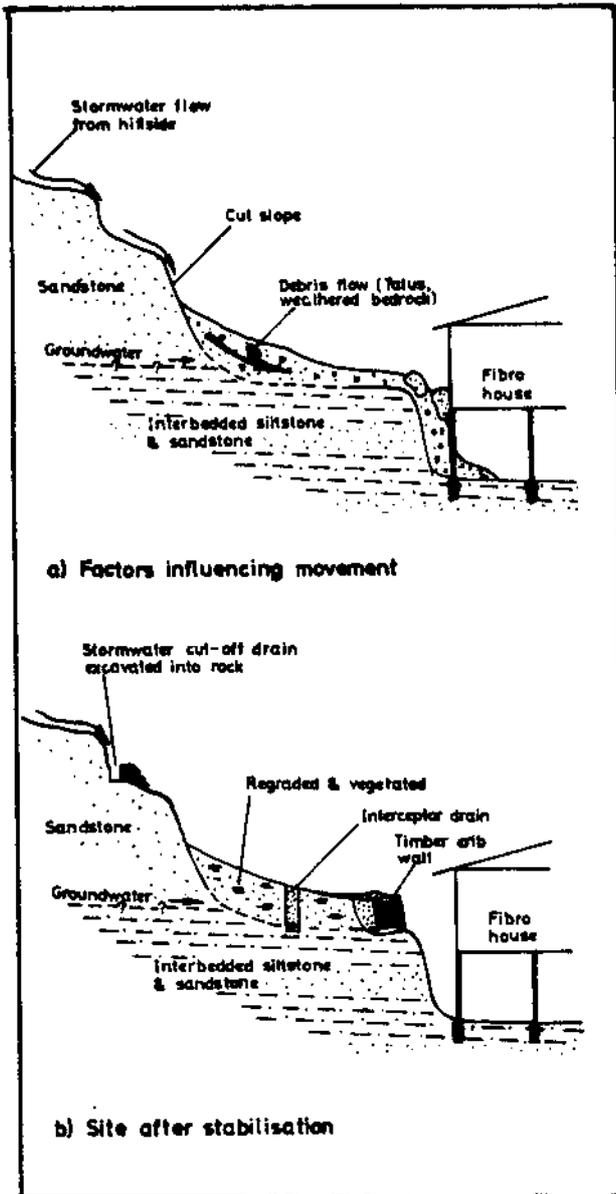
Figure No.10 - Umina Earthflow
