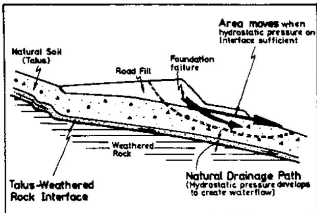
Figure No.7 - Slide Mechanism Devils Elbow
