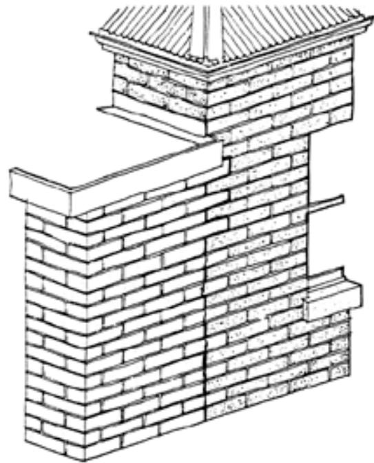
Figure 8: Cracking to an addition
