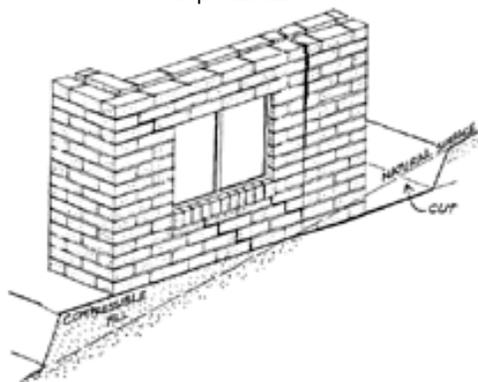
Figure 7: Cracking due to cut and fill
