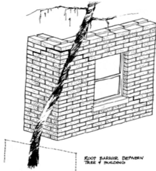
Figure 3: Cracking due to tree damage
