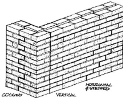
Figure 1: Types of Cracking
