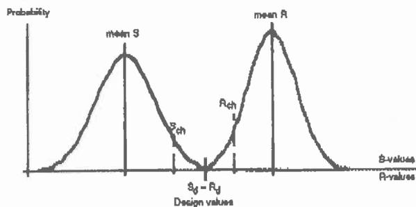
Figure 3. Distribution of action values and material properties
